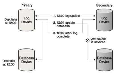
Figure 56. Data inconsistency caused by a rolling disaster
