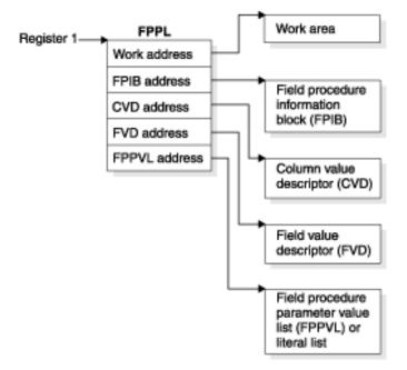
Figure 72. Field procedure parameter list
