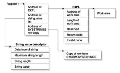
Figure 71. Pointers at entry to a conversion procedure
