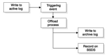
Figure 37. The offloading process
