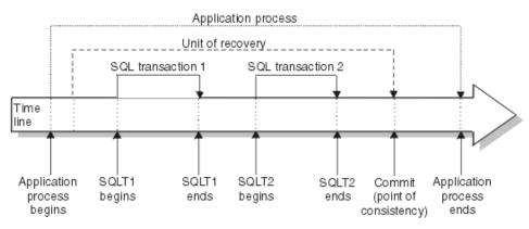
Figure 35. A unit of recovery within an application process
