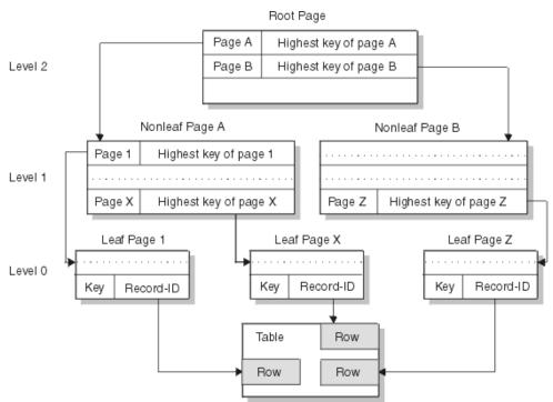
Figure 18. Sample index structure and pointers (three-level index)
